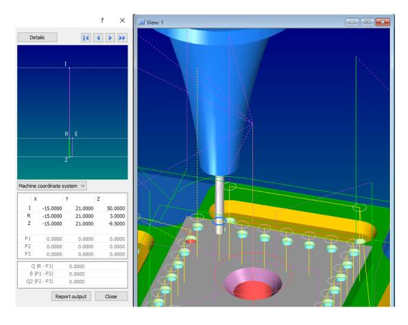
• Position of initial point, return point, bottom of hole, etc., depth of cut, amount of clearance
